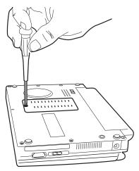
Sample unscrewing the memory module slot cover
